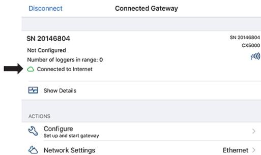
If you need to set up Ethernet for static IP addresses or WiFi, tap Network Settings and tap Ethernet or WiFi.
