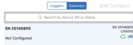
If the gateway does not appear, make sure it is powered up and within range of your phone or tablet or press the button on the gateway.
