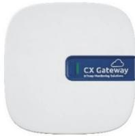
The InTemp CX5000 Gateway is a device that uses Bluetooth® Low Energy (BLE) to regularly download up to 50 CX series loggers and upload the data to the InTempConnect® website automatically via Ethernet or WiFi. The gateway requires an InTempConnect website account with gateway privileges and a phone or tablet with the InTemp app to set up the gateway.
