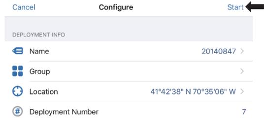
Logging will begin based on the settings you selected. See *Deploying and Mounting the Logger* for details on mounting and see *Reading Out the Logger* for details on downloading.
