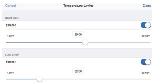
6. Enable Low Limit if you want burst logging to occur when the sensor reading falls below a specific reading. Drag the slider to the reading that will trigger burst logging or tap the value field and type a specific reading. In the example, the logger will switch to burst logging when the temperature falls below 32°F.
