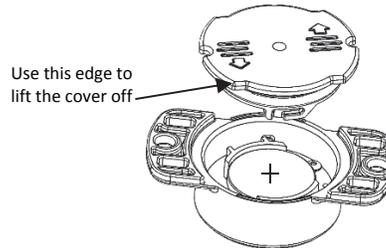
3. Remove the battery and place a new one in the battery holder, positive side facing up. Use a small flat-head screwdriver to carefully pop the battery out of its holder as shown.
