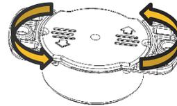
2. Use the edge below the arrow on the cover to lift it off the logger.
