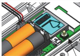
Install the rechargeable batteries. Press this button on the mote for 3 seconds.
