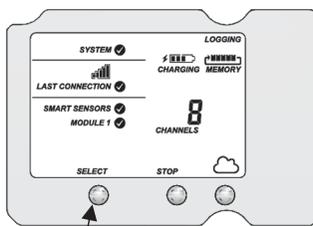
Press the Select button on the RX3000 station to switch to the module where the RXW Manager is installed (Module 1 or Module 2).
