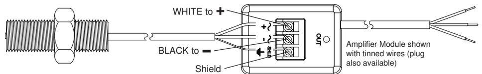
Figure 2 Magnetic Sensor to Amplifier Connection Detail
