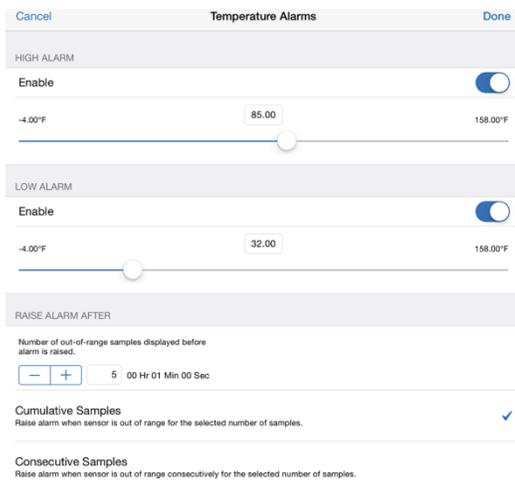
5. Enable the Low Alarm if you want an alarm to trip when the sensor reading falls below the low alarm value. Drag the slider to the reading that will trip the alarm or tap the value field and type a specific reading. In the example, an alarm is configured to trip when the temperature falls below 32°F.
