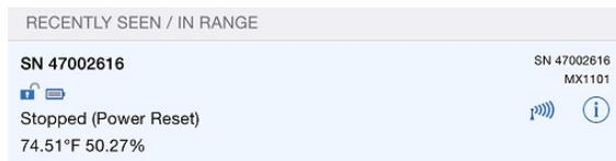
Tap the row in the list to connect to the logger. If it does not appear in the list, make sure the logger is within range of your mobile device. Note that current sensor readings are always visible in this list even if the logger is not logging.
