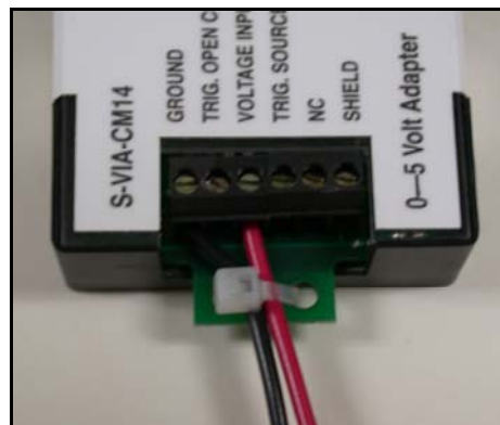
Figure 1: Cable strain relief
