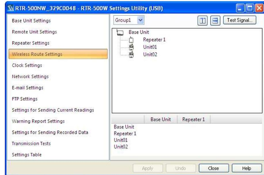
There is something else shown in this 2<sup>nd</sup> screen that is very interesting and useful. That is the results of the Signal Strength Test. Clicking on the Test Signal button will cause the system to perform an RF signal strength test for all registered communication paths and display the results. In this case we can see that all routs are 5 / Green, which is as good as it can get.
