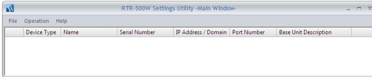
2. Next connect the RTR-500NW/AW to your PC using the USB cable supplied with the unit. If the USB driver installed correctly the software should automatically discover the 500W, and the device will appear in the Utility Main Window. If this doesn't happen automatically you may have to manually associate the USB Driver with the 500W in your PC's Device Manager.
