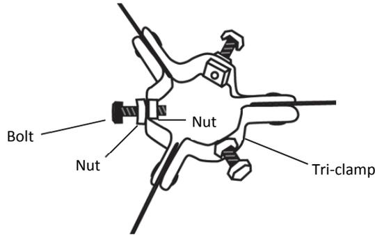
3. Install the remaining five nut and bolt assemblies in the same manner for both upper and lower tri-clamps. Make sure the bolt assemblies on the upper and lower mast tri-clamps leave enough room for the lower mast section to slip through.
