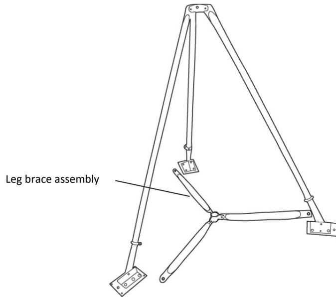
8. Attach each of the three inner legs to each of the leg U-bolt assemblies (5/16-18 inch) using the inner stud of the U-bolt. To attach each inner leg, remove the nut from the inner stud, slide the leg over the stud, and then tighten the nut finger tight.
