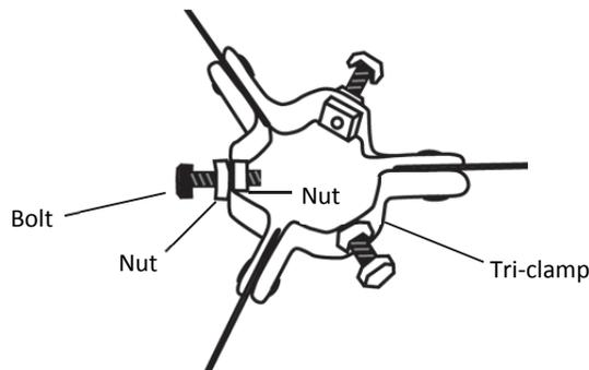
4. Install the remaining five nut and bolt assemblies in the same manner for both upper and lower tri-clamps. Make sure the bolt assemblies on the upper and lower mast tri-clamps leave enough room for the lower mast section to slip through.
