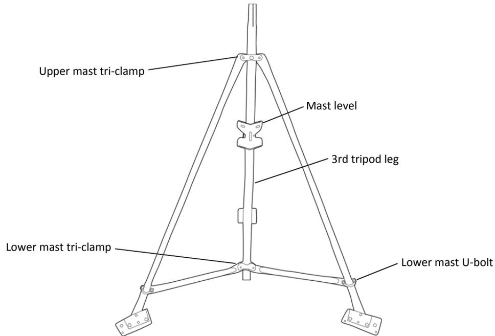
10. Install the mast level (M-MLA) on the lower mast as shown in the previous figure.
