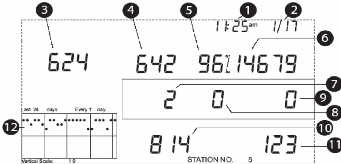
1. Time of day or the number of times the anemometer reed switch was seen closed\*. The reed switch opens and closes once each revolution of the anemometer. Press the WIND key to toggle between these two values.
