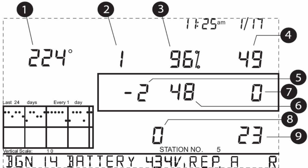
1. 8-bit timer value of next reception.\* The degree sign displaying in the upper right hand corner next to this value verifies that the Reception Diagnostic screen is currently displayed.
