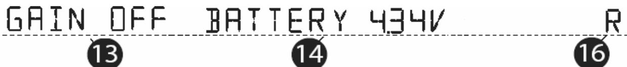
13. The Receiver Gain setting provides control over the receiver sensitivity. Press HI/LOW to toggle Gain on and off. If you're having trouble with reception, try changing the Gain. Note that Gain can adversely affect performance depending upon conditions. If you are having reception problems, you should try both settings. Gain should generally not be turned on when signal strength is above 30. See #4 below. Gain setting is automatic for later firmware versions.
