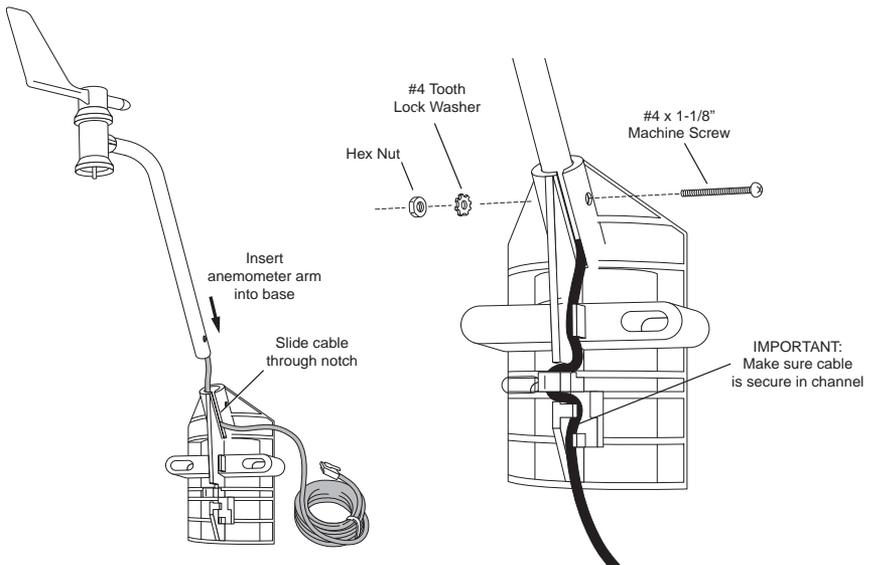
4. Slide the tooth-lock washer and hex nut onto the machine screw. Tighten the hex nut while holding the screw with a Phillips head screwdriver to prevent it from turning.
