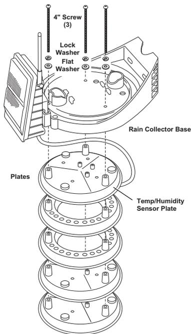
Note: For some models of the ISS, the order in which the five radiation shield plates are assembled may be slightly different than the order shown in the figure on page 25. For this reason, ensure that you always reassemble the plates in the same order in which they were disassembled.
