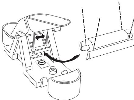
**Open plastic arms to insert metric measurement adapter,
