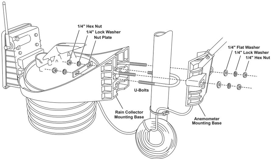
If you wish to put the anemometer higher than the rain collector side of your ISS on the support tube, follow the instructions in the ISS Installation Manual for mounting each side *separately*.
