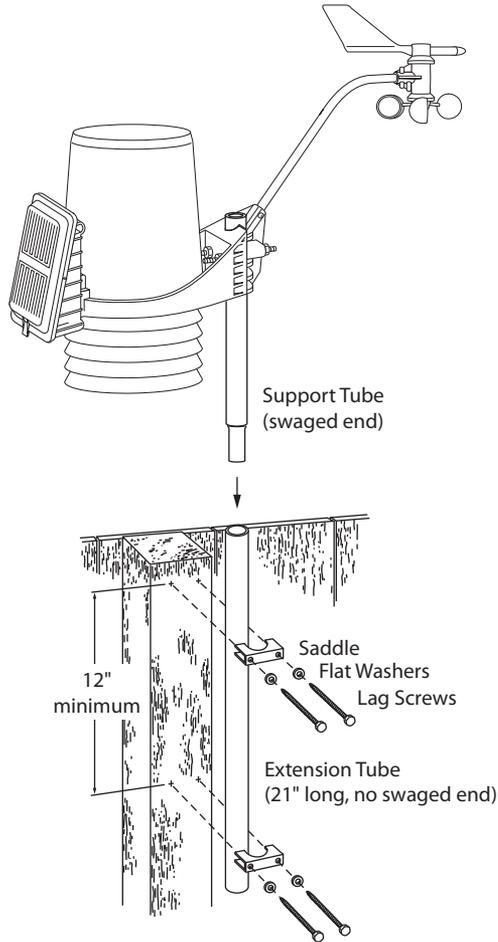
4. Tighten the lag screws until the tube will not slide up or down no matter how hard you try to move it.
