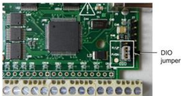
Figure 5. Pull-up/down jumper location
